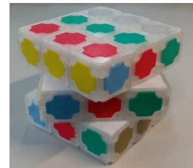
全3D列印零件組裝之魔術方塊 Rubik's cube consisting of all 3D printed PLA parts
