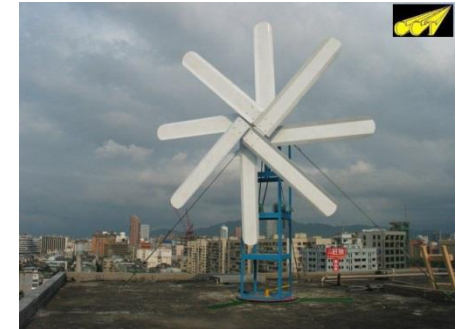
風力製冰與發電兩用機 Dual System of Wind Chiller Integrated with Wind Generator
