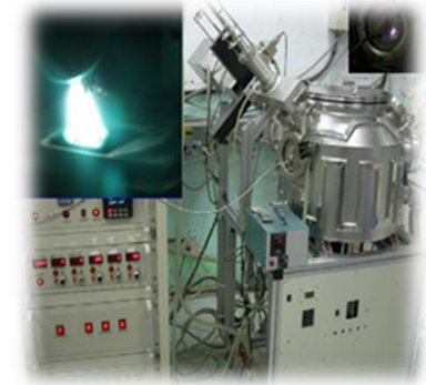
人造鑽石薄膜製程 Processes of Diamond Films Fabrication
